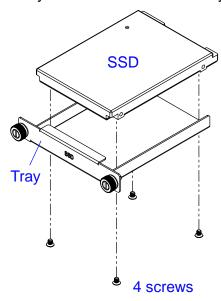
3. Put and secure the tray back to the device.
