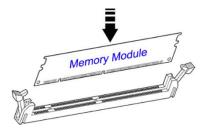
To remove the module, press the ejector tabs outwards with your fingertips to eject the module.
