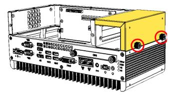
2. Remove the expansion slot fillers by releasing the two screws below.
