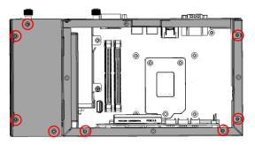
Then release the 4 screws below to take out the bracket.
