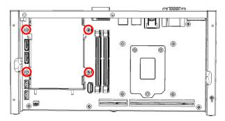
3. Install the 2<sup>nd</sup> SSD onto the bracket, secure it with 4 screws as pointed by arrows below.
