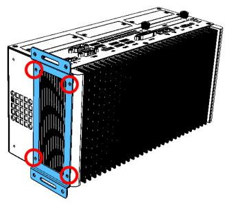
2. Prepare at least 4 screws (M3) to install the device on wall .
