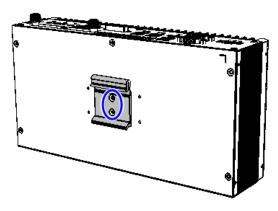
Secure with 4 screws for a rotatable bracket.
