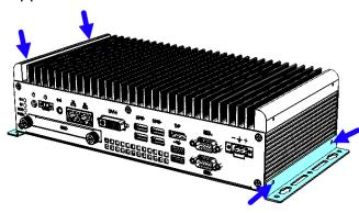
2. Prepare at least 4 screws (M3) to install the device on wall .
