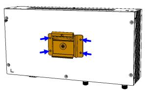
2. Hook the DIN rail mounting bracket over the top of the DIN rail, and then press the lower section of the bracket towards the DIN rail to clip the bracket onto it.
